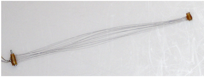
Fig. 2 Picture of the SMA wire bundle actuator.
