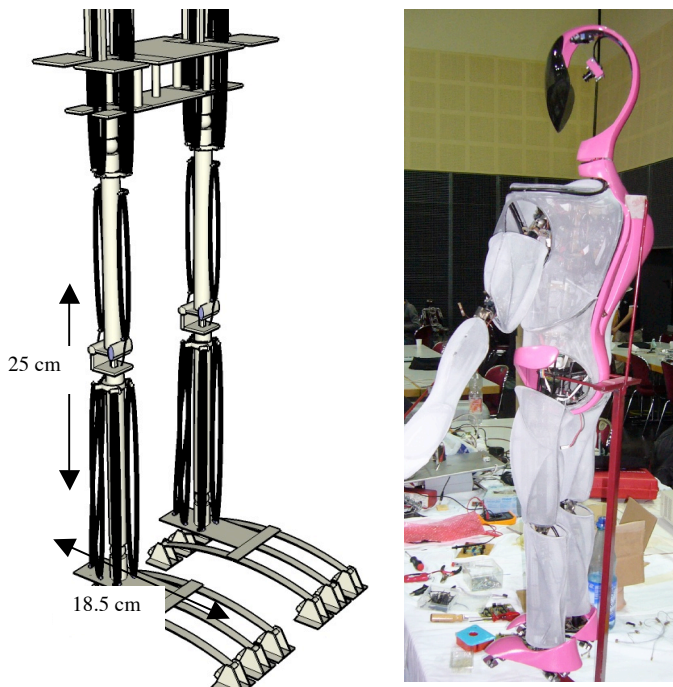
Fig. 3 Picture of the humanoid robot Lara actuated by SMA muscles and CAD-model of the legs.
