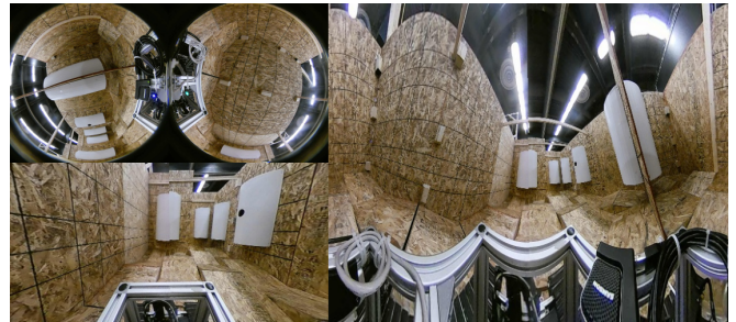
Fig. 1: Two fish-eye images are streamed from the omnidirectional camera (top-left), which are converted to perspective (bottom-left) and Mercator projection (right).
