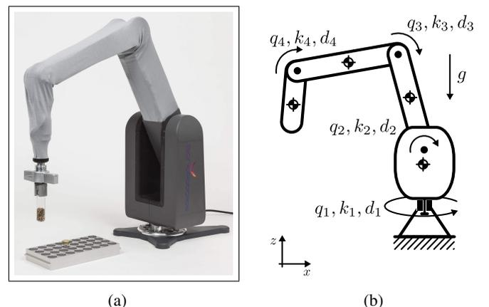
Figure 5: Picture (a) and schematic diagram (b) of the elastic robot arm BIOROB X4 (Bionics Robotics, Germany).
