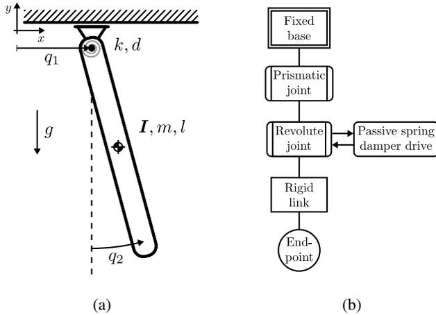
Figure 2: Schematic diagram (a) and model tree (b) of the pendulum on trolley.
