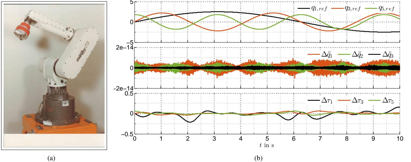
Figure 4: Picture (a) and simulation results (b) of the robot arm MANUTEC R3 (manutec, Germany) given in SI units.
