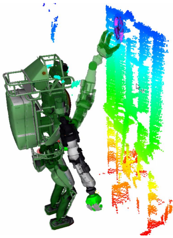
Fig. 8 Operator view of the experiment setup. The operator has requested point cloud data of the environment and the Valve Template (purple) has been located to match the sensor data of the real valve. The Atlas robot is unable to reach the valve as shown by the green ghost robot used for previewing the target arm motions.
