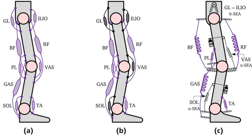
**Figure 3: Evolution of BioBiped1's actuation concept: (a) human musculoskeletal leg system; (b) selection of actuators and passive elements: the hip joint requires both active flexion and extension, while in the knee and ankle joints only actuated extensor muscles are required (highlighted); c) implementation of passive and active elements as motors and springs [23].**
