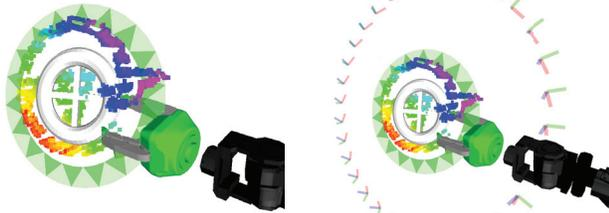
(c) Valve template overlapped with steering wheel pointcloud. (d) Circular path of the wrist.
