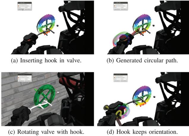
Fig. 2: Simulation experiment to turn a valve 360 degrees.
