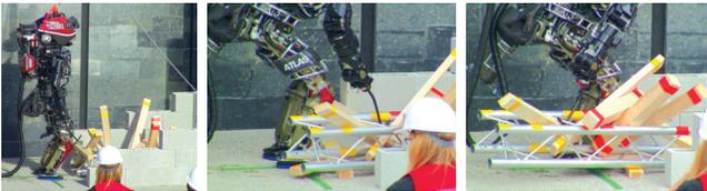
(a) Robot and truss. (b) Grabbing the truss. (c) Truss being pulled.
