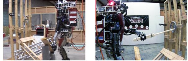
(a) Valve blocked by debris. (b) Reaching valve with stick.
