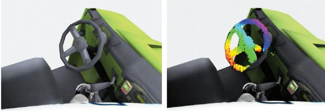
(a) Robot view of a steering wheel. (b) Pointcloud of steering wheel.
