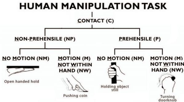
Fig. 5: Manipulation classification to be used in our approach. Image based on [25].
