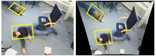
Fig. 3. Original image taken by quadrotor at the height of 1.77 meters (left) and ground plane projection (right). The shown rectangles correspond to ground truth annotations.
