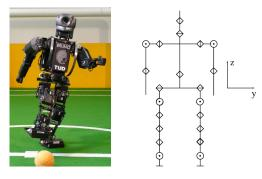
Autonomous humanoid robot *Bruno* kicking a ball (left, with designed head) and kinematical structure of the robot (right).
