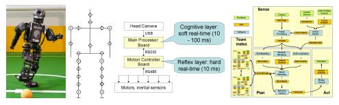
**Fig. 1.** Autonomous humanoid robot *Bruno* (with designed head) kicking a ball (left), kinematical robot structure (middle left), main layers of information processing (middle right) and control architecture (right).
