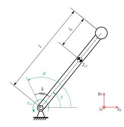
Fig. 3. Principle of a BioRob joint [4]
