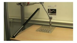
Fig. 6. Execution of a pick-and-place application [11]
