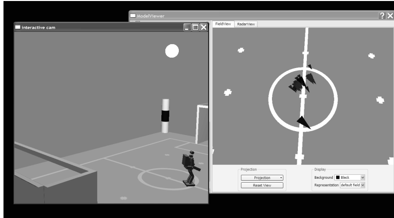
Fig. 7. Interactive testing of self localization. Left window: Interactive simulation. Right window: The data provided by the self-localization software (red arrows depict particles, dark blue arrow is pose estimate) can be compared to the robot's position and direction in the simulation (sole blue arrow).
