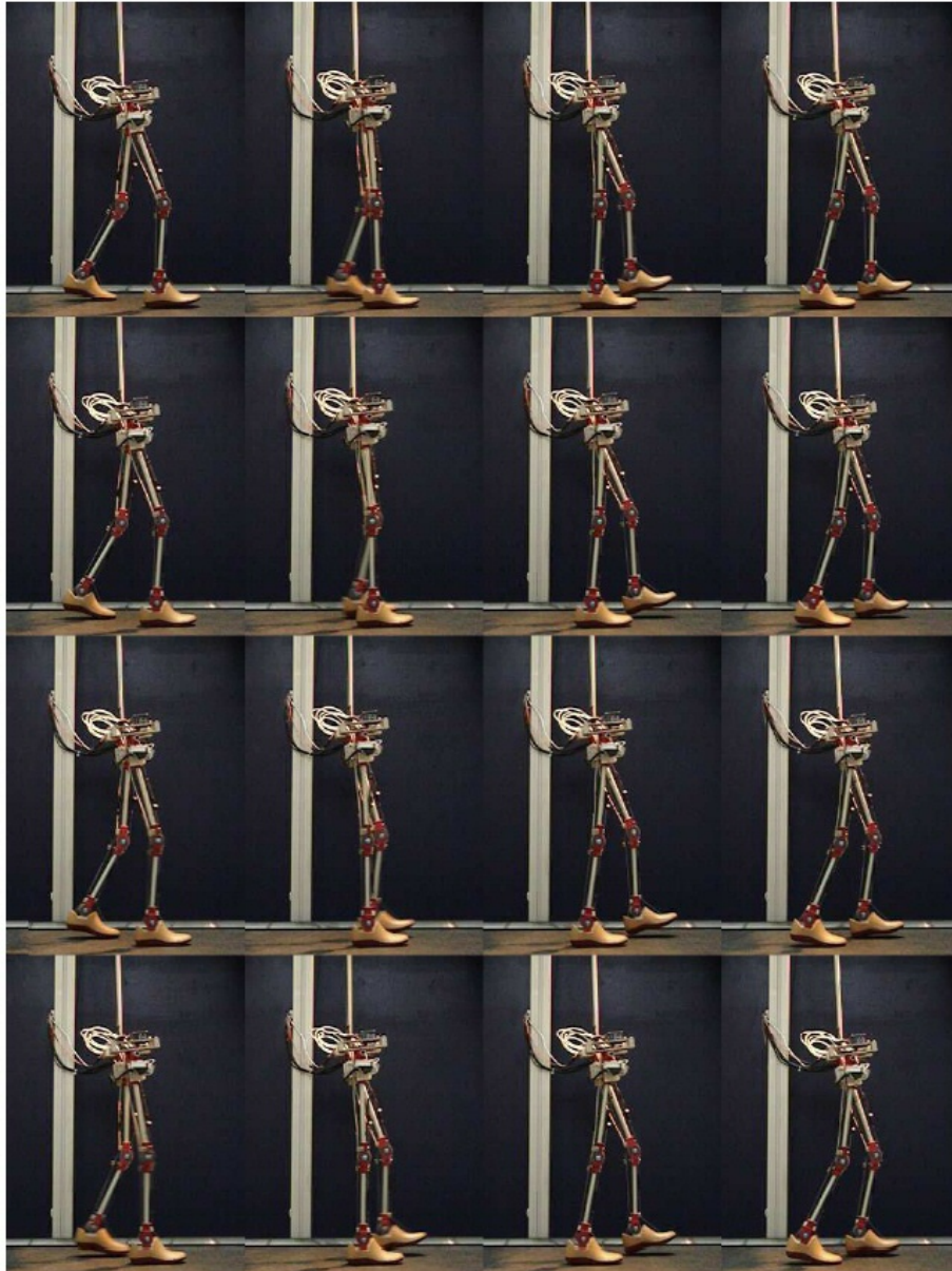
Figure 3: Walking sequence of JenaWalker II at moderate speed.
