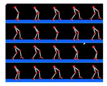
Fig. 10. Bipedal walking with passively compliant three-segmented legs: Resulting gait sequence for parameter set optimized for low hip torques and bounded minimum walking speed (page 12).
