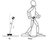
Fig. 3. The inverted pendulum model is used as a simplified model to describe walking properties of humanoid robots and humans.
