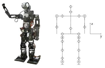
Fig. 1. The 55 cm tall, autonomous humanoid robot Bruno developed at TU Darmstadt (left) and its kinematic structure with 21 servo motor driven joints (right).
