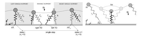
**Fig. 4.** A basic compliant leg model exhibits properties of both human-like walking (left) and running (right) in the same mechanical design (due to [Gey05]).
