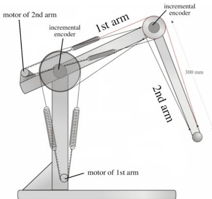
Fig. 3: Design principle of the bionic manipulator (2 DOF).
