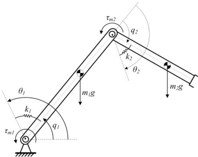
Fig. 1: 2 DOF rotational manipulator with series elastic actuation. The elongation of the elastic elements is defined by the difference between link position  $q$  and motor position  $\theta$ .
