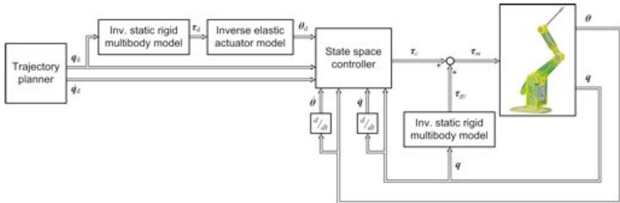
Fig. 4: Control structure of the BioRob manipulator.
