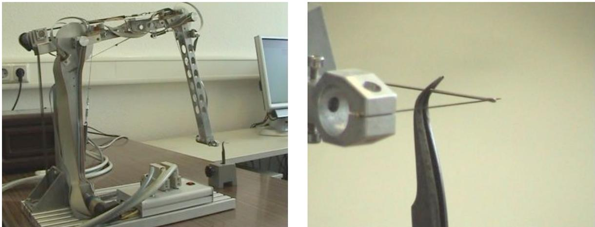
Fig. 6: Experimental setup demonstrating the repeatability characteristics of the manipulator.
