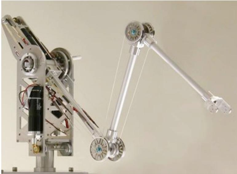
Fig. 2: Mechanical setup of the new 4 DOF demonstrator with a range of 1 m.
