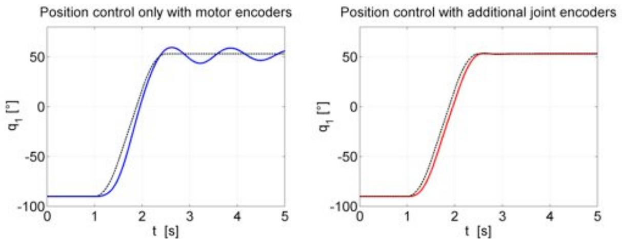
Fig. 5: Position control of the first link of the 3 DOF elastically actuated manipulator (obtained in simulation).
