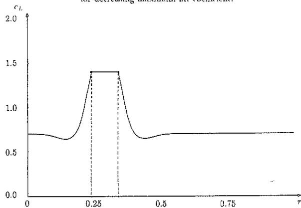
Fig. 13. Lift coefficient versus normalized time; optimal trajectory.
