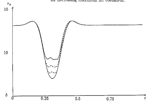
Fig. 11. Horizontal velocity component versus normalized time for decreasing maximum lift coefficient.
