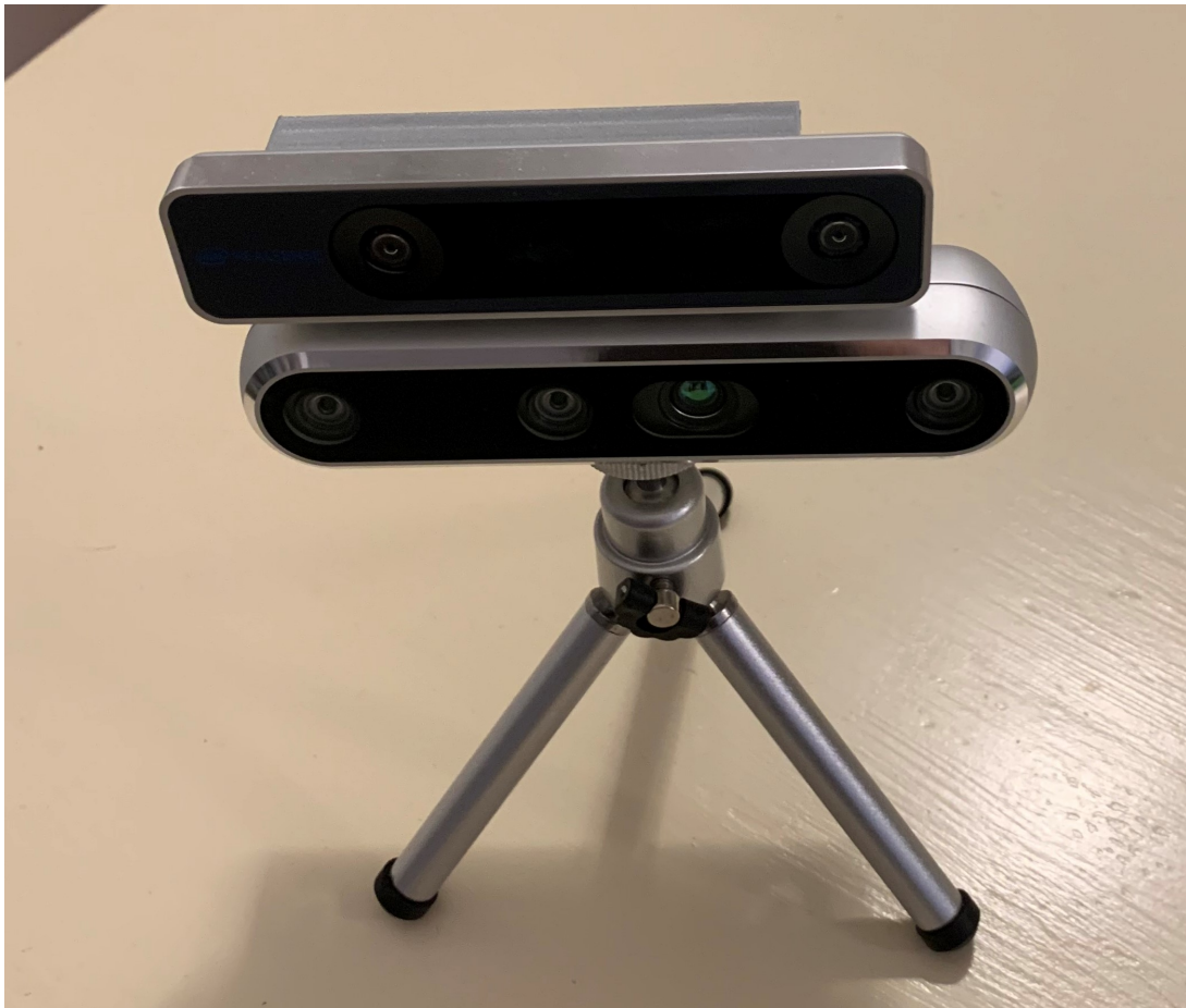
Figure 6.6.: Camera setup consisting of a D455 depth camera [9] and a T265 tracking camera [32].
