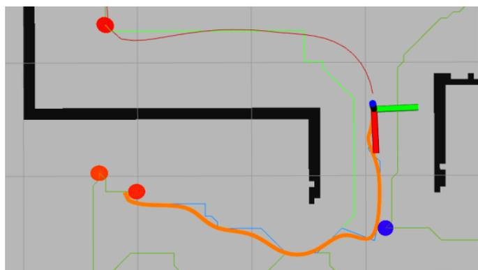
Figure 6.11.: Updated path during execution. The axes show the current position of the robot. The light green line is the original planned path, the blue one is the updated path. The thick orange line is the smoothed one. The dark red line is the trajectory already driven.
