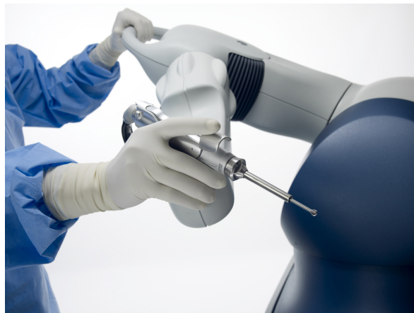
Figure A.2.: Handheld arm of the MAKOPlasty RIO [52]
